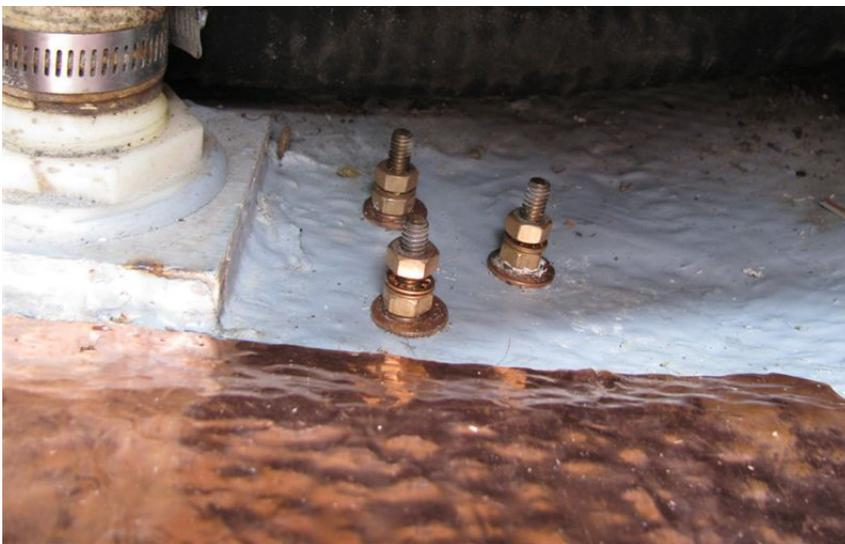
Here are the bronze bolts connecting to the external ground plane immersed in sea water. One can directly connect the ground foil to the bolts (by sandwiching the foil between two lock washers), or if galvanic corrosion protection is needed, then a galvanic isolator can connect the bolts to the ground plane.
